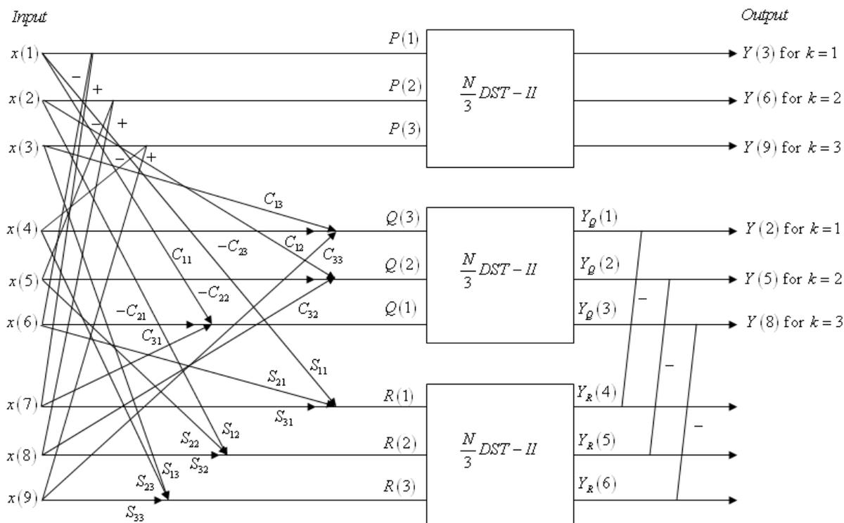
Figure 3: Signal flow graph for realization of the output components  $Y(2)$ ,  $Y(3)$ ,  $Y(5)$ ,  $Y(6)$ ,  $Y(8)$  and  $Y(9)$  of radix-3 DST-II of length  $N=9$ .
