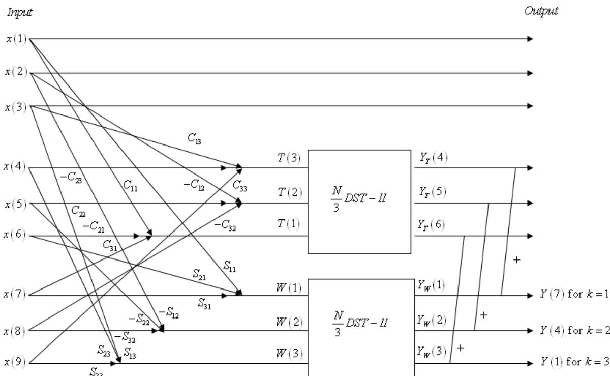
Figure 4: Signal flow graph for realization of the output components  $Y(1)$ ,  $Y(4)$ , and  $Y(7)$  of radix-3 DST-II of length  $N=9$ .
