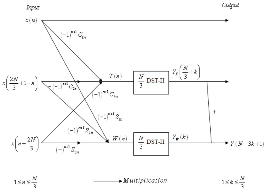
Figure 2: Block diagram for realization of output components  $Y(N-3k+1)$  of radix-3 DST-II of length  $N$ .
