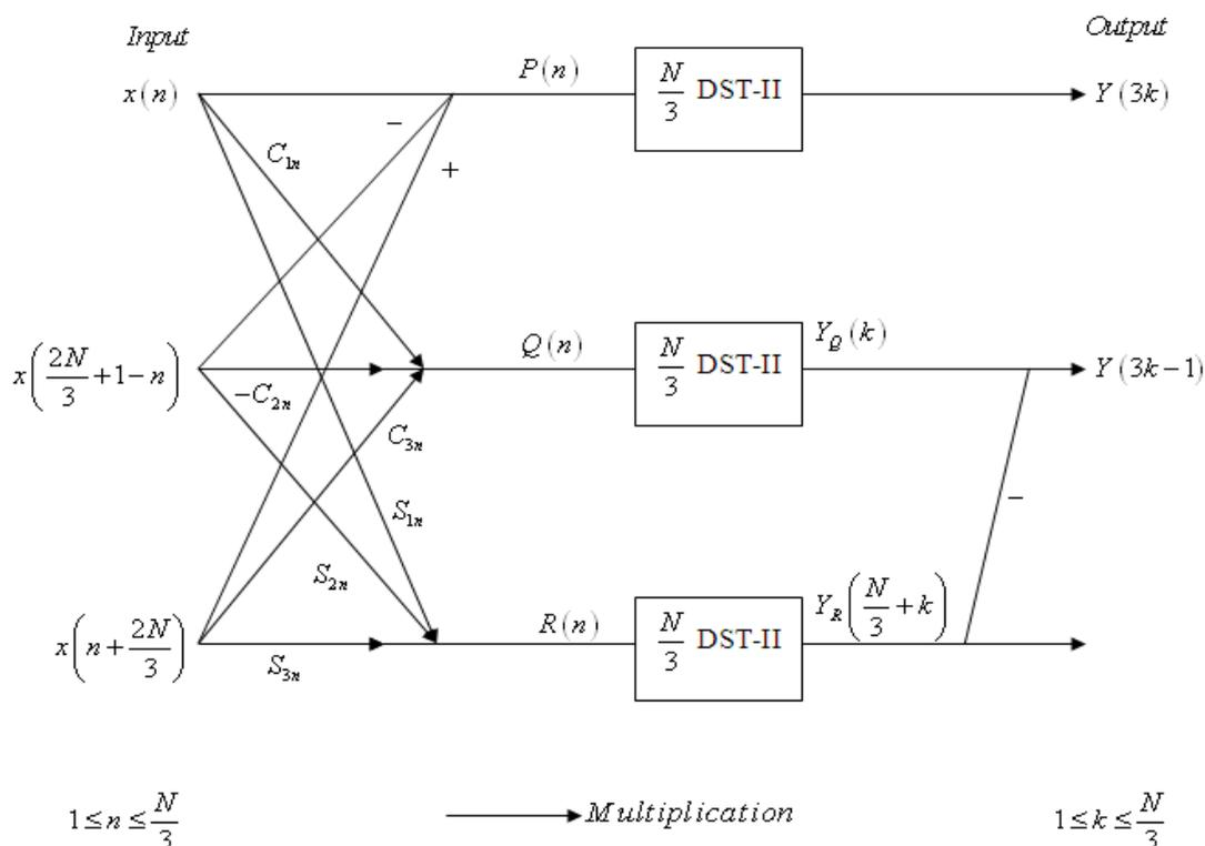
Figure 1: Block diagram for realization of output components  $Y(3k)$  and  $Y(3k-1)$  of radix-3 DST-II of length  $N$ .
